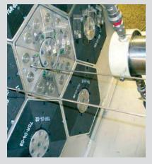
Preparation for the measurement of the neutron field in a model of part of the transmutor under development with fluoride salt-based fuel. The target chamber of the neutron source can be seen on the right-hand side of the photograph.
