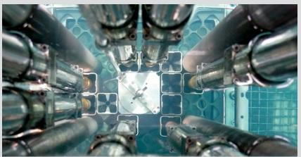
Preparation of the active zone for a basic critical experiment to be carried out in the "Vrabec" educational reactor at the Faculty of Nuclear Sciences and Physical Engineering of the Czech Technical University in Prague. The active zone comprises a module containing fluoride salts.
