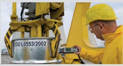
Dosimetric inspection of waste to be accepted at the repository.
