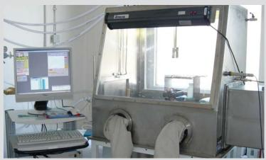
Experimental equipment for studying electrochemical characteristics at the Nuclear Research Institute at Řež – nickel electrolyser installed in dry box.
