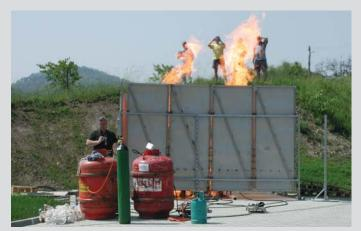
Testing of a waste container burning test facility.
