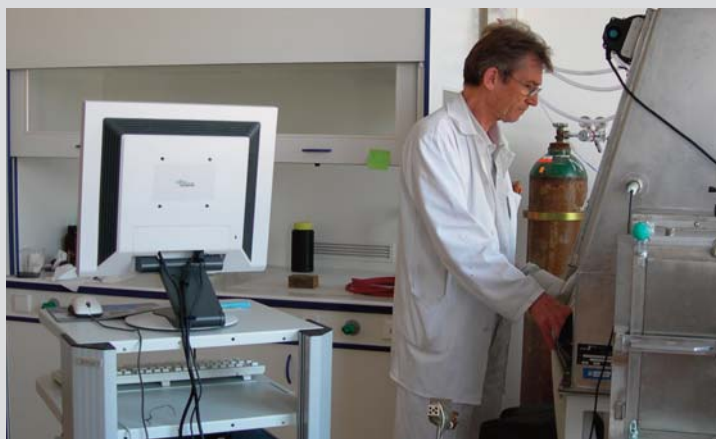
A dry box with a nitrogen atmosphere.
