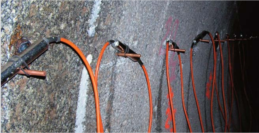
Bedřichov gallery - an experimental underground workplace operated by the Liberec Technical University; geophysical resistance measurement instrumentation placed along the gallery wall.
