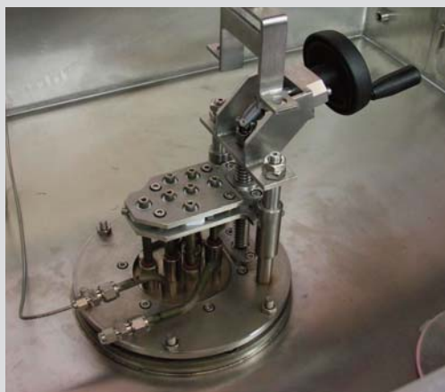
A flange equipped with a movable system designed to grip an electrode set used for electrochemical measurements in fluoride melts.
