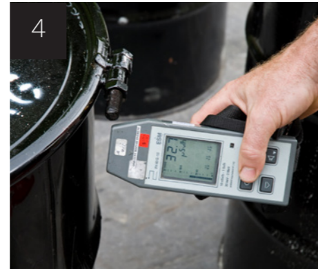
4 Control measurements are taken of the activity and weight of individual packages
