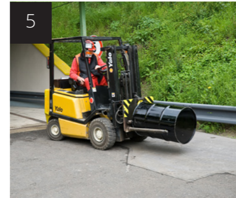
5 The waste packages are then transferred to the underground disposal area
