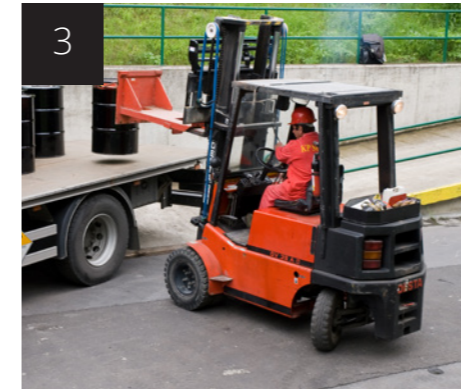
3 The waste packages are removed one-by-one by fork-lift truck
