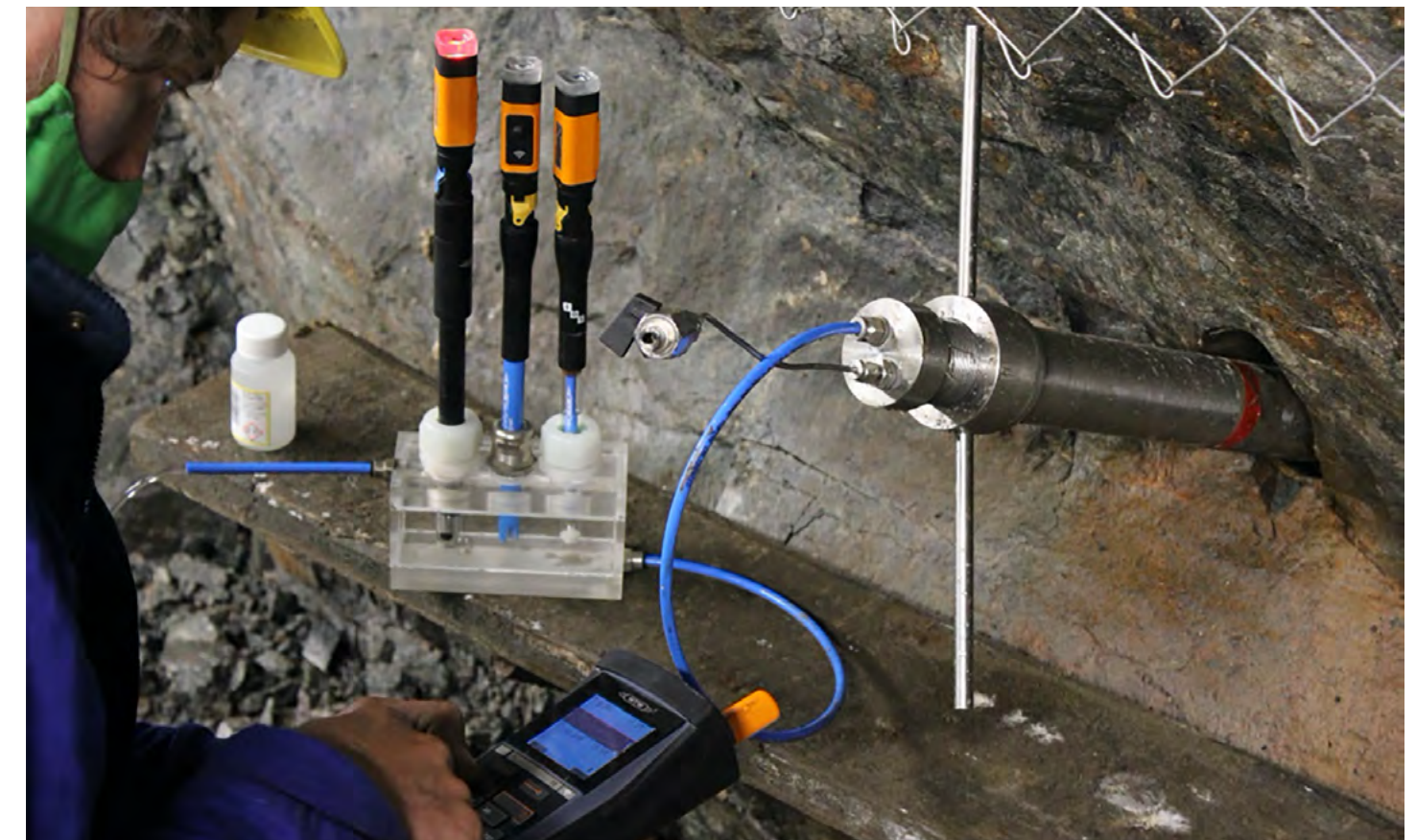
↑ Geochemical measurements in the pilot borehole S-27
