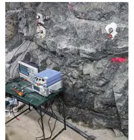
↑ Testing of seismic measurement equipment at the Bukov URF
