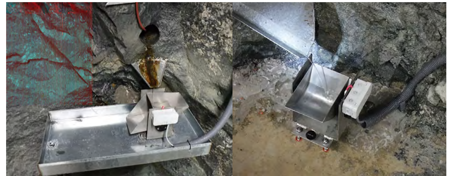
↑ System for the measurement of water inflows to the Bukov URF employing tilting vessels
