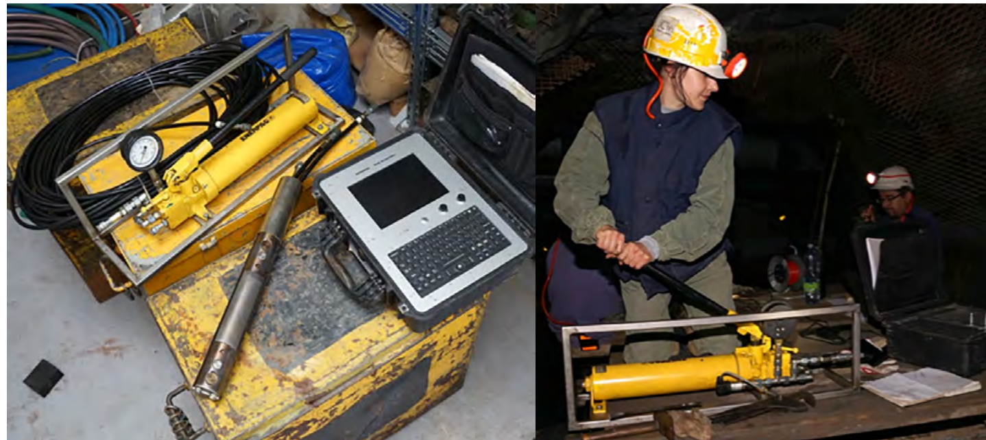
↑ Goodman Jack device for the measurement of rock deformation properties
