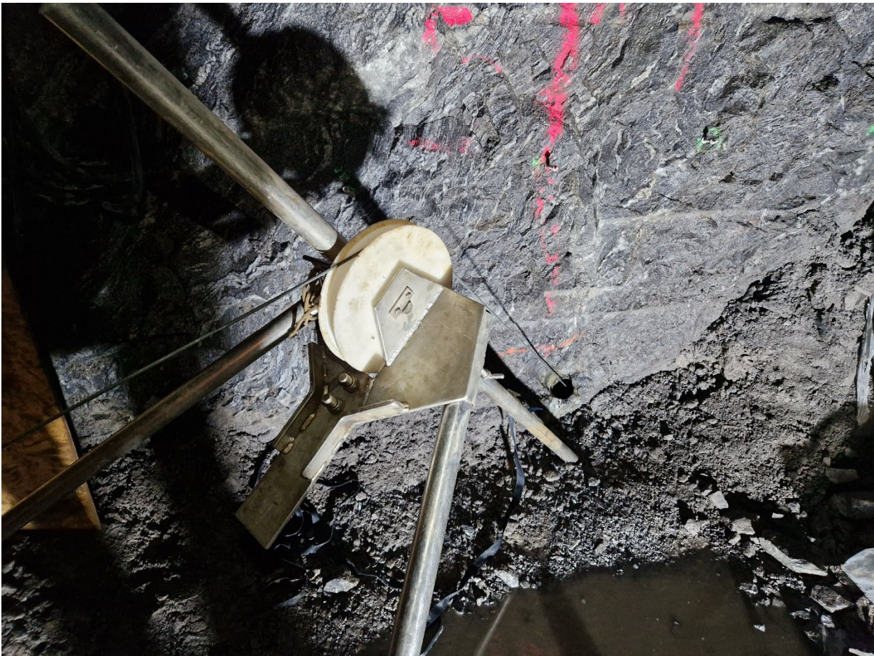
Figure 4. Borehole L8-54DL and the wheel used for guiding the cable from the winch into the borehole.
