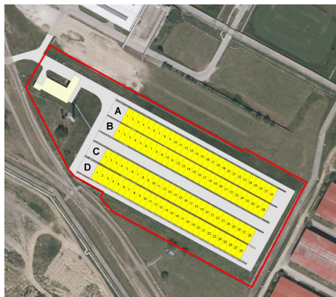
Fig. 18 Layout of the Dukovany repository showing the double rows of disposal chambers
