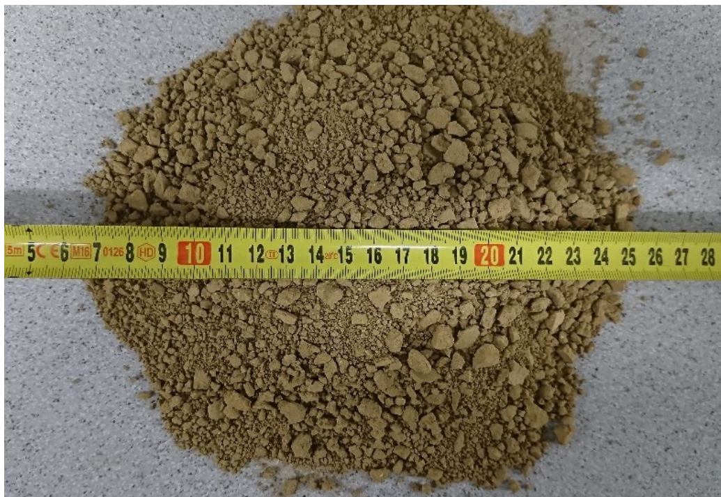
Fig. 14 Bentonite pellets from the final compression tests (Pacovský et al. 2018)
